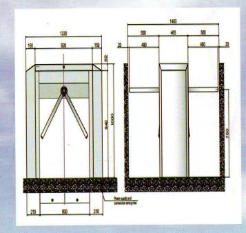
The **MOSFi** TT-910 (DUAL WAY BIDIRECTIONAL TRIPOD TURNSTILE) designed to ensure the pedestrian access control aesthetically thanks to the incorporation of two tripods mechanisms in only one housing. Furthermore, it reduces overall dimensions and infrastructure works needed for the implementation thereof: time of installation, electrical wiring of power supply and connection, etc.
